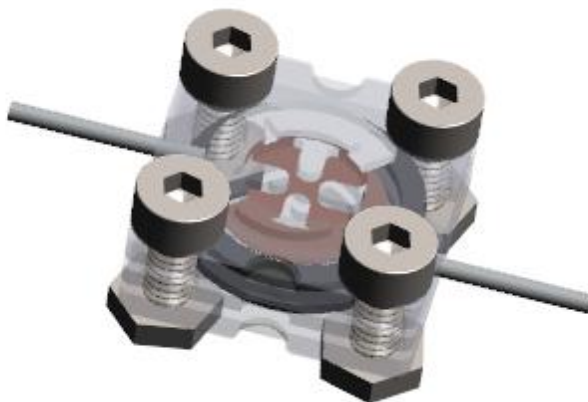
Figure 10. Test rig for sensor membrane flow experiments. The two tubes on the left and right hand side is the inlet and outlet respectively. The sensor membrane is fixated with sealing tape on a holder which again is clamped between the transparent top and bottom cover plates. Also visible on the drawing is the four lugs pointing towards the centre which provide mechanical support for the membrane.
